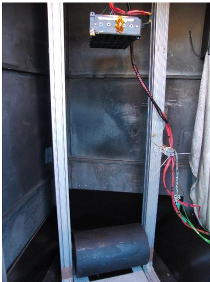
Figure 30: Drop testing setup according to FreedomCar and experimental data, Hybrid Commercial Vehicle (HCV) project.
