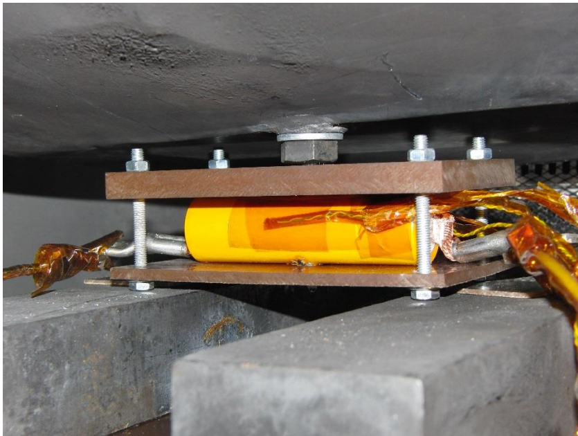
Figure 31: Cylindrical cell in test-frame during nail penetration test.
