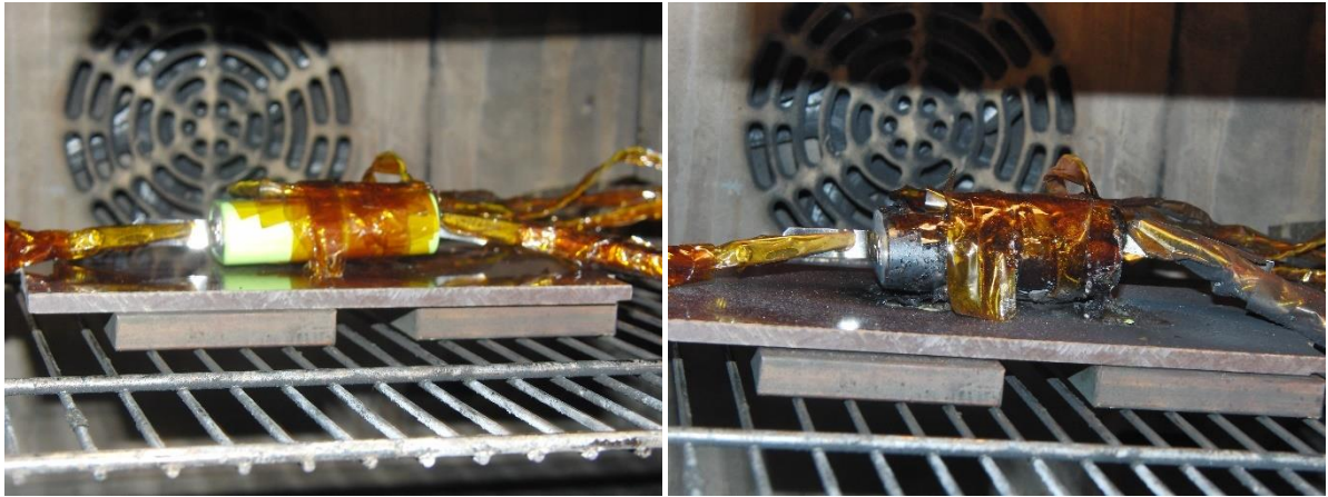
Figure 35: Test setup for a thermal stability test, and photo of the same setup after the test.
