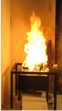
Figure 34: Example picture of a fire test of lithium-ion batteries performed at RISE Research Institutes of Sweden. In this example, the pouch cells were mechanically tightened together using steel wires and placed on a wire gratings with a propane burner underneath.
